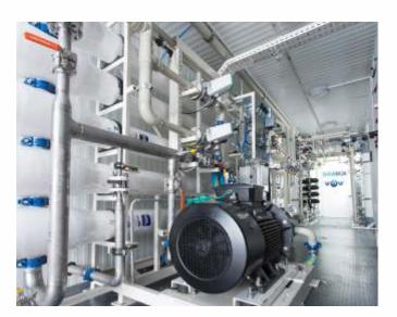
WOWs units are self-contained and includes filtration, ultra filtration, pumping equipment, membranes, electrical controls, and chemical feed and control components to operate the entire range of treatment solutions from pre to post-treatment and can be operated and monitored using smart technology.
